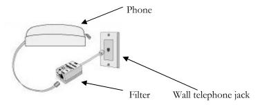
One form of filter is a splitter, which has one male plug and two female jacks. This lets you use the same phone jack for
